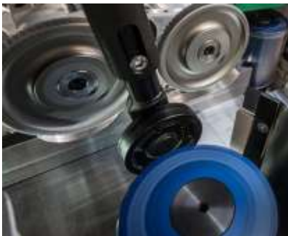
Pressure roller from above located opposite the left spindle pivoting out of the way, spring loaded.
