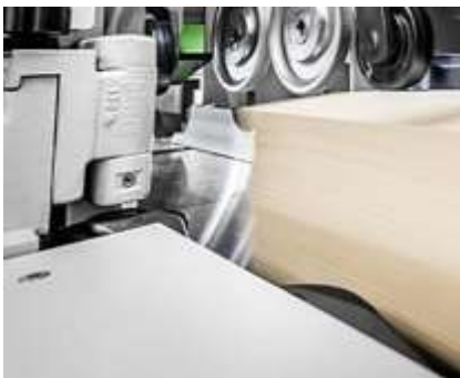
Two lateral roller pressure in front of left spindle revolving and spring-mounted
