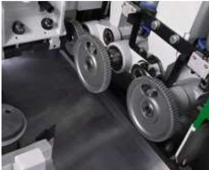
Setting range of the feed rollers opposite left spindle, axial 35 mm
